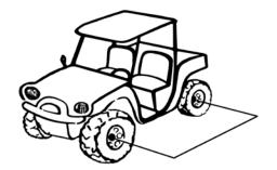
Wheelbase is the distance between the center of the front axle and the center of the farthest rear axle
